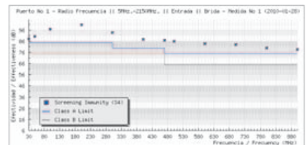
Screening of the male IEC connector ref.413201
